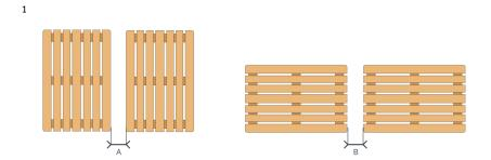
Any payload overhang increases the dimensions by the size of the overhang.
