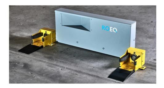
ROEQ DS500 docking station is designed for ROEQ S-Cart500 Ext and S-Cart500W. The DS500 solution comes in two versions: **Active** and **Passive**. DS500 Active locks carts in place via electromagnets, ensuring maximum stability during loading and unloading of carts. DS500 Passive holds carts in place with no lock function.
