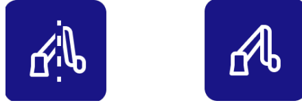
Fig. 2.3: The dashed line going through the manipulator joystick button shows that the arm is not currently in safe home.
