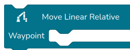
Fig. 3.30: The Move Linear Relative block per default contains one Motion instruction but can contain several.
