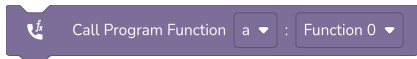
Fig. 2.28: The Call Program Function block has a field to select a program and a function.
