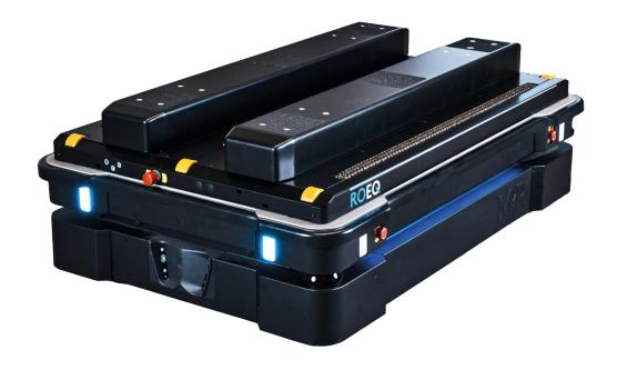
The ROEQ Lift 'n' Roll provides a unique dual-functionality solution, enabling efficient pallet handling between pick up & drop-off stations, such as pallet racks and conveyor stations. One of the key advantages is that it interacts directly with conveyor stations – eliminating the need for split conveyors, optimizing valuable factory floor space and simplifying the installation.
