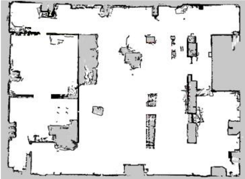
Figure 4.5 Example of a floor plan that includes too much noise and too many dynamic obstacles
