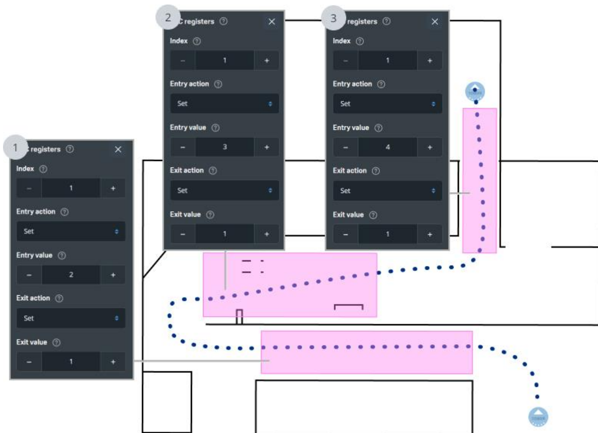
Figure 4.17 A map where I/O module zones are used to affect which solution is applied in each area
