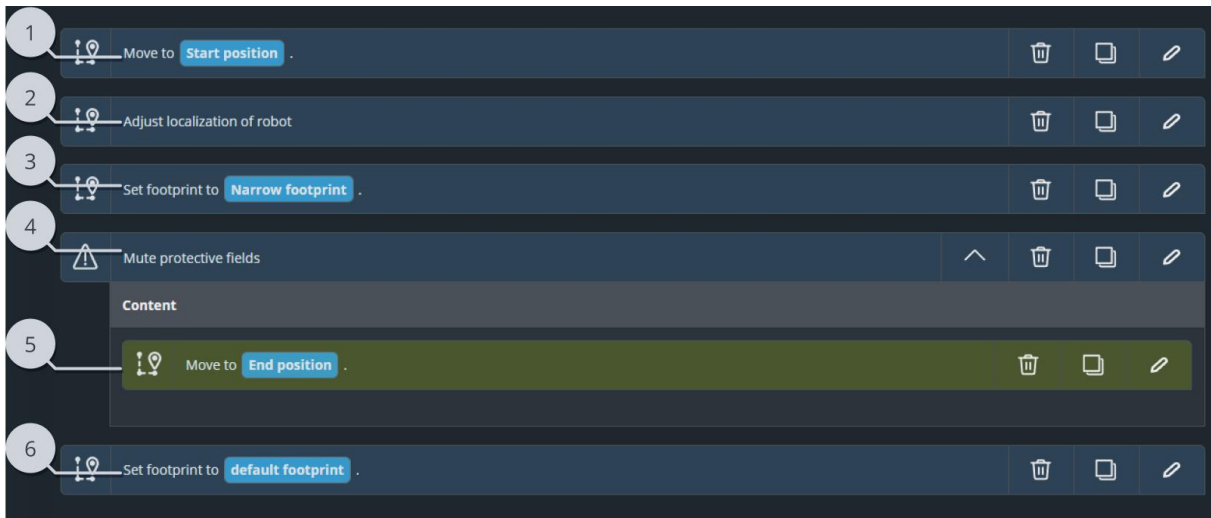
Figure 4.7 A mission to send the robot through narrow gaps
