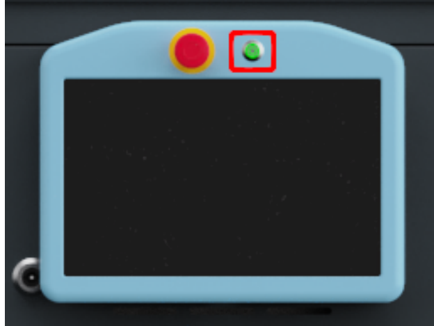
Fig. 4.11: UR power button is located to the right of the emergency stop
