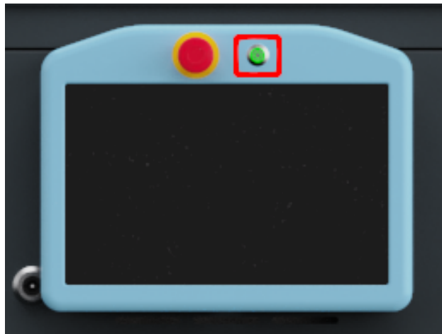
Fig. 4.2: UR power button is located to the right of the emergency stop
