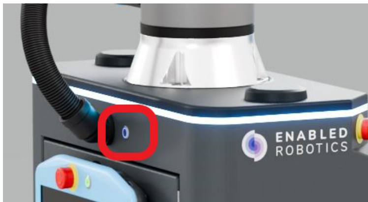
Fig. 4.4: The reset button is located on the rear of the robot
